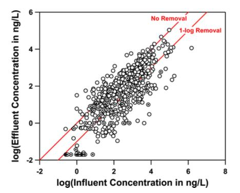
Comparison plot of pharmaceuticals and personal care products effluent concentration as a function of influent concentration for WWTPs utilizing traditional treatment operations (i.e., solids removal and CAS-conventional activated sludge)
